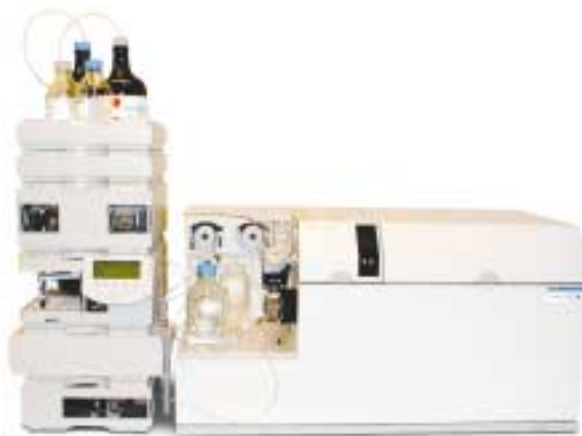
LC-ICP-MS combines the 1100 Series LC with the 7500 ICP-MS.
